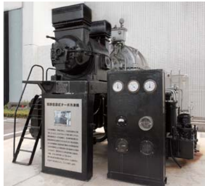
1930 Takasago and Ebara-type centrifugal refrigerating machines, which was Japan's first refrigerating machine
