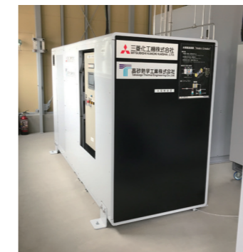
Water electrolyzer delivered to the demonstration site in Noshiro
