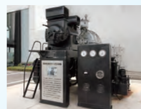
1930 Takasago Ebara turbo refrigerator, which was the first domestically-produced product
