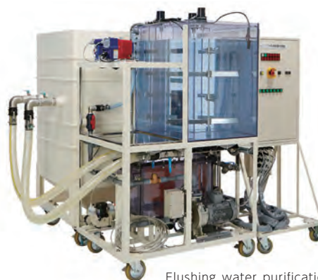
Flushing water purification unit
