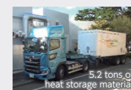
5.2 tons of heat storage material Heat transport by trailer
