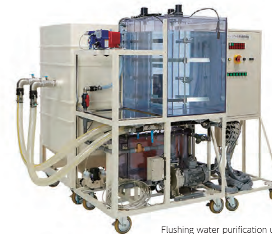
Flushing water purification unit
