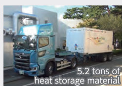
Heat transport by trailer 5.2 tons of heat storage material
