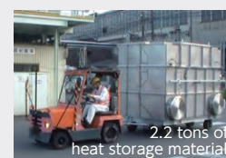
Heat transport by in-plant vehicle 2.2 tons of heat storage material
